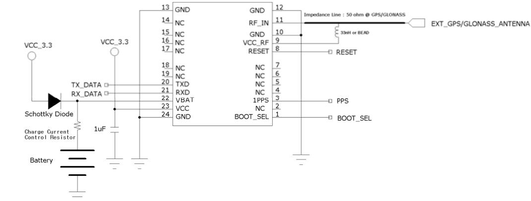
2. Example 2 for GPS/GLONASS External Active Antenna
