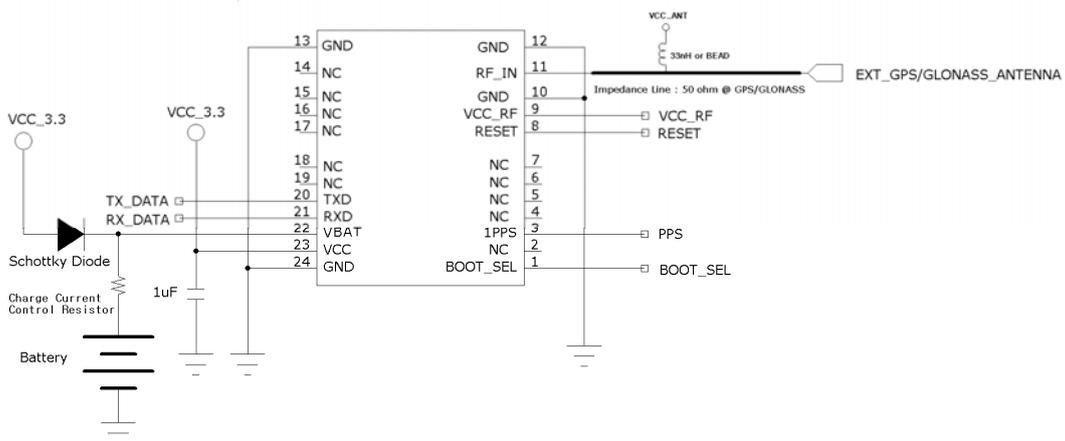
3. Example 1 for GPS/GLONASS Patch Antenna
